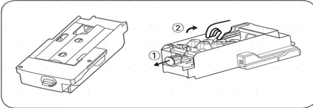
4. After cleaning the tray, put it back in, then firmly push in the icemaker, close the freezer drawer, and switch on the icemaker function via the display panel.
